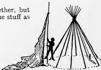
3 rd Set up tenth pole with teepee cover fastened to it by lash-rope.
